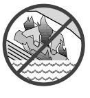
Do not operate if any portion of the heater was submerged in water or if any corrosion occurs. Immediately call a qualified service technician to inspect the appliance and to replace any part of the control system and any gas control that has been under water.
