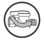
**WARNING**: Prior to removing the glass, shut off gas to the appliance (or remove the batteries from the battery box and shut off electricity to the fireplace). This prevents any chance of accidental burner ignition when accessing the firebox.
