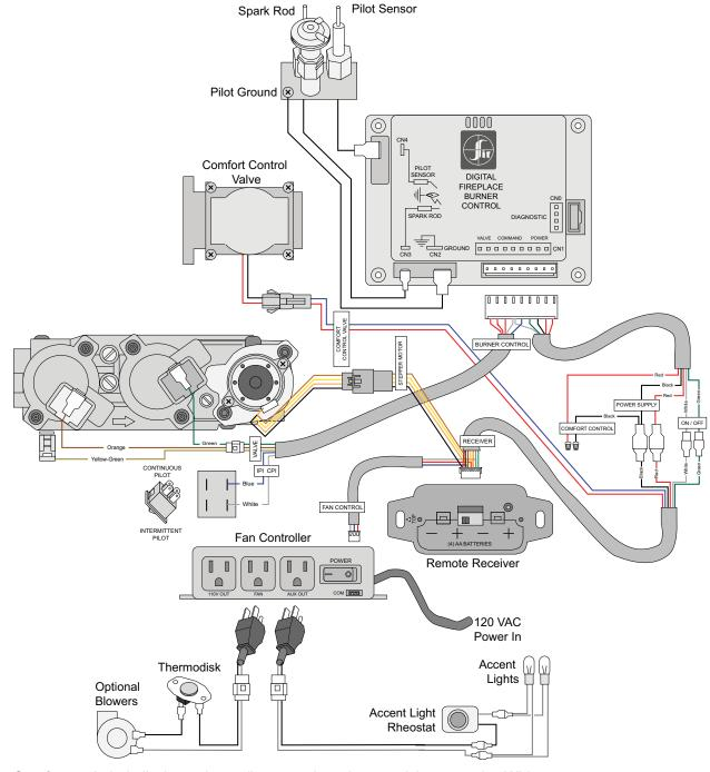
**<u>Caution</u>**: Label all wires prior to disconnection when servicing controls. Wiring errors can cause improper and dangerous operation.
