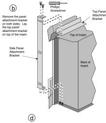
Position the side attachment bracket, with side panel attached, onto the insert. Make sure the tab on the insert inserts into the rear noton the side attachment bracket. Repeat this step for the opposite side. Attach the top panel attachment bracket with the four screws removed in step "b".
