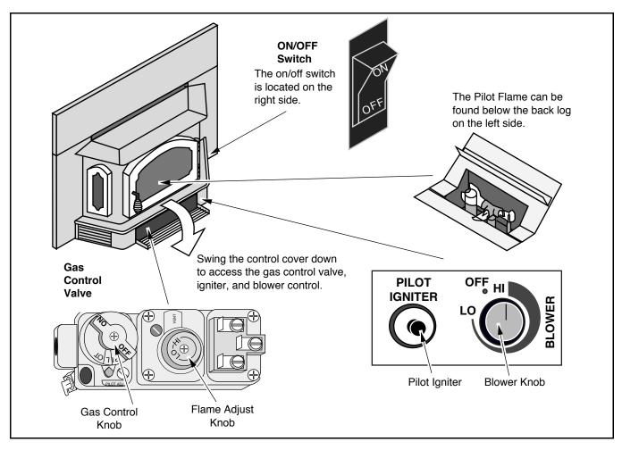
**Blower Knob** This knob controls the speed of the internal convection blower that pushes the
