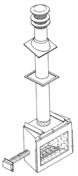
THIS FIREPLACE IS U.L. LISTED FOR USE WITH THE "L" SERIES CHIMNEY SYSTEM COMPONENTS.
