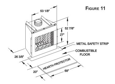
WARNING: THE HEARTH EXTENSION AND THE METAL SAFETY STRIP SHOULD BE INSTALLED ONLY IN A HORIZONTAL RELATIONSHIP TO THE FIREPLACE, AS ILLUSTRATED.
