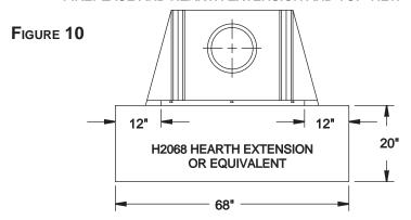
NOTE: A hearth extension placed on a combustible floor must be constructed with rigid insulation which has a minimum "R" value of 1.16 or a "K" value of 0.43. The insulation must be covered with a non-combustible covering such as a tile stone, marble, or a piece of 0.018 minimum sheet metal which is needed to protect the insulation. Follow instructions provided with the fireplace for all other specifications and directions for proper installation of the fireplace and hearth extension.
