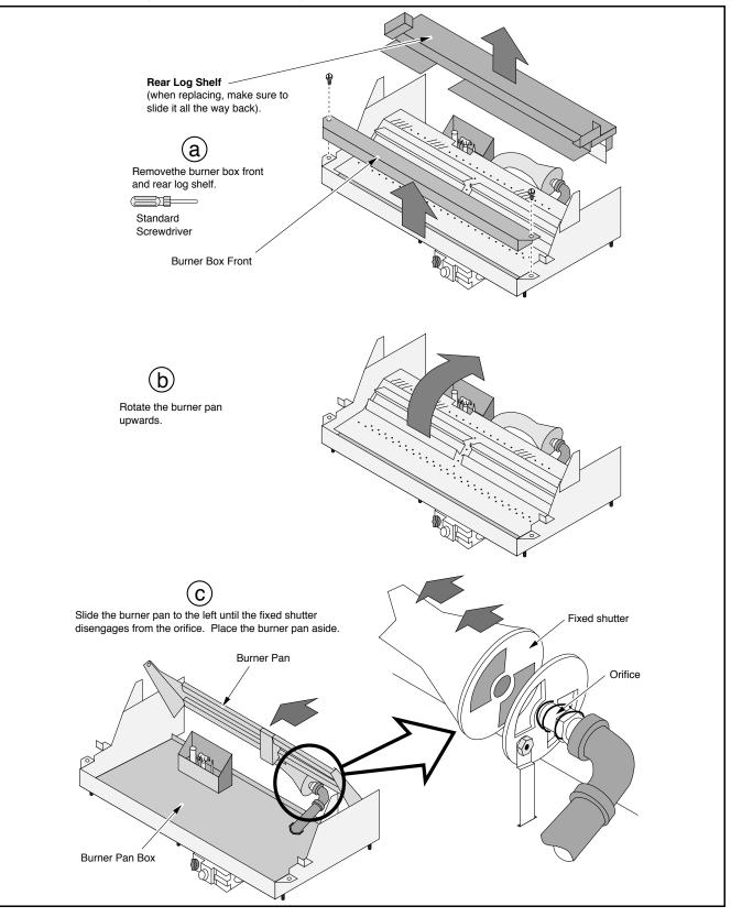
**3** Follow the directions below to remove the natural gas orifice. Apply thread sealant to the LP orifice (#49 - it has "49" stamped on it) and tighten in place with a 1/2" open end wrench. Replace the spring. Slide the adjustable shutter back in place.
