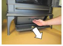
2. Slide the ashpan forward. Use the built-in handle to pull the ashpan out of the firebox.
