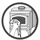
Maintain the door and glass seal and keep them in good condition. Do not operate this heater with broken or missing glass.
