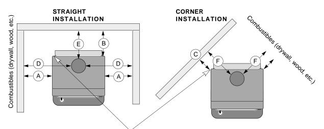
NOTE: Measure rear clearances from the edge of the stove top, not the rear heat shield.
