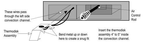
3 Install the wire clip following the directions below.
