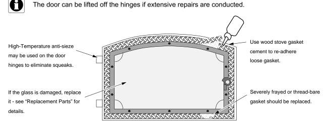
The door latch should pull the door against the face of the stove (but not so tight as to not allow full handle rotation). If the latch requires adjustment, follow the directions below.
