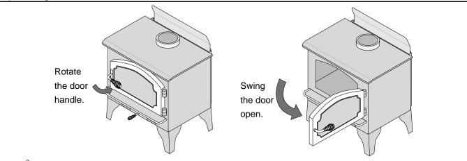
The door becomes hot during use. Use a glove to open the door if the handle is hot.
