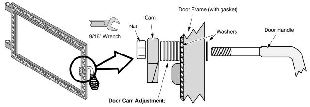
To tighten the door cam, remove the door handle and discard one of the washers betwen the door frame and cam. To loosen the door cam, add a washer between the door frame and cam.
