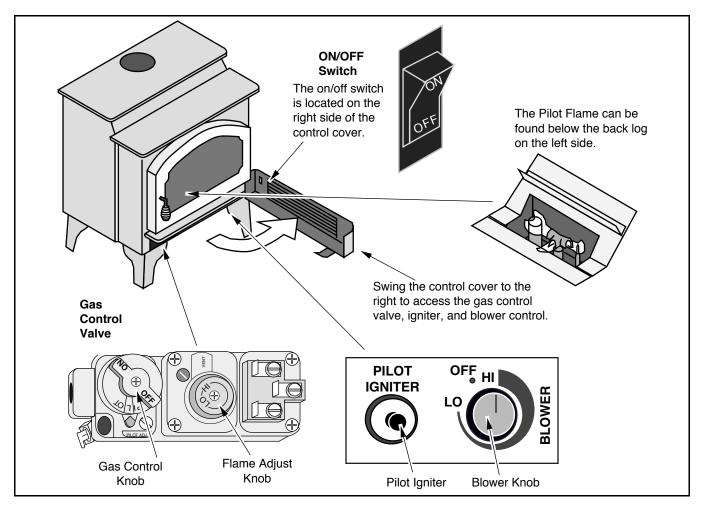
**Blower Knob** This knob controls the speed of the internal convection blower that pushes the heated air into the room.
