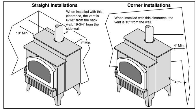
+ Clearances may be reduced by methods specified in NFPA 211, listed wall shields, pipe shields, or other means approved by local building or fire officials.
