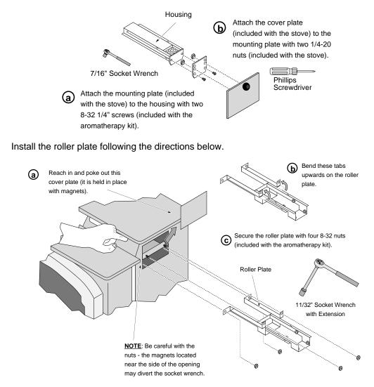
3 Slide the housing into the roller plate following the directions below.
