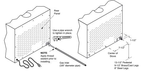
A manual shutoff valve is required for installation (it must be located within 3' of the heater).). T-Handle
