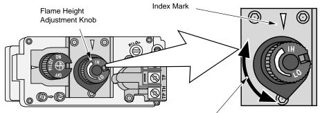
Turn counter-clockwise to adjust the flame higher, clockwise to lower.
