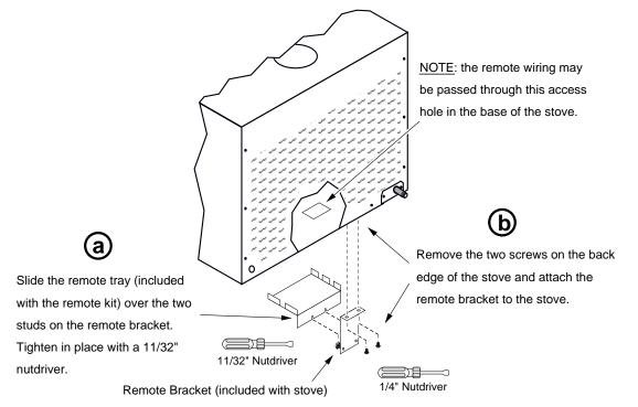
2 Place the remote reciever into the bracket as shown (the wires are routed below the stove, in front of the control cover).
