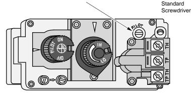
The pilot flame must contact the thermocouple and thermopile (see the illustration below). Adjust the pilot up or
