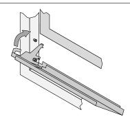
Swing the grill upwards to engage the upper slot. You will need to lift the grill slightly to get it over the bushing. Once in place the grill is held in place by gravity.
