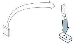
Remove the bulb from the socket as shown above.
