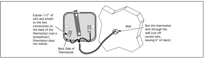
4 Pull the cover off the thermostat. Place the thermostat in location and attach it to the wall through the two obround holes (use the appropriate screws for the type of wall it is being attached to). Replace the cover on the thermostat to complete the installation.
