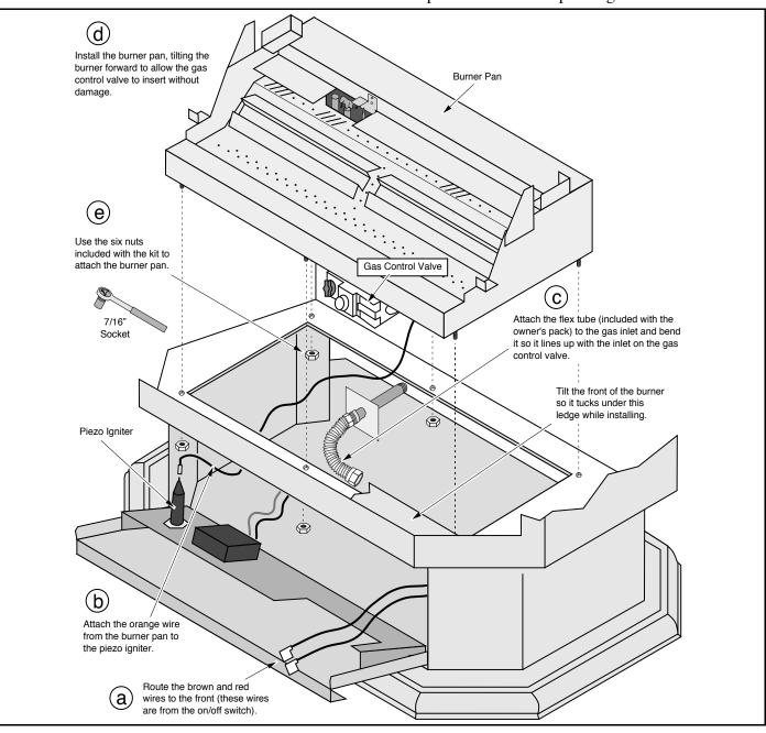
**d** Follow the directions below to install the burner pan and attach the piezo igniter wire.
