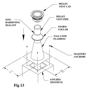
the Storm Collar will go. Slip the Storm Collar down over the pipe, and affix it to the pipe with a 1/4"-long stainless steel sheet metal screw. (Figures 13 & 14). The Storm Collar will then support the entire vent system. Install the Cap. Seal the joint at the Storm Collar, and any other joints or seams which may appear suspect. Figure 15 show a Tall Cone Flashing modified to fit a chimney where the tile liner protrudes
