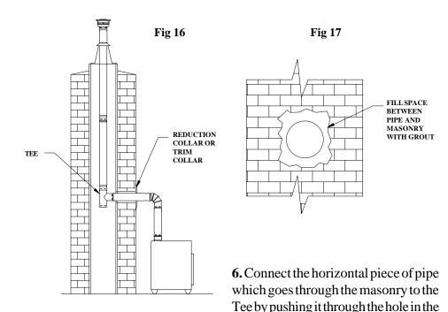
masonry, and lining it up with the branch of the Tee. Then push it into the Tee, while twisting to lock it.
