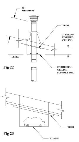
Adaptor. Using a level, make slight adjustments in the position of the appliance until the pipe is truly vertical. Tighten the bolts in the Clamp. Note that the overall length of the pellet vent pipe as assembled, can be no longer than 42 feet.
