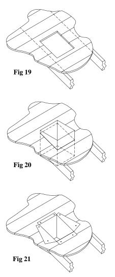
centered on the small hole which you drilled through the ceiling to mark the location. Again, insure that you are not cutting through rafters or framing members.
