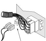
Attach the quick-connects to the two posts near the molex connector on the circuit board (orientation does not mater).
