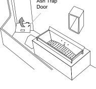
(d) Slide the ash pan trap door forward to expose the ash dumps (the door can be removed and cleaned if necessary)
