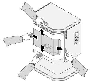
When properly adjusted, the door should be evenly spaced from the front of the stove (and shut tight, compressing the gasket).
