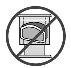
The viewing door and ashpan must be closed and latched during operation.
