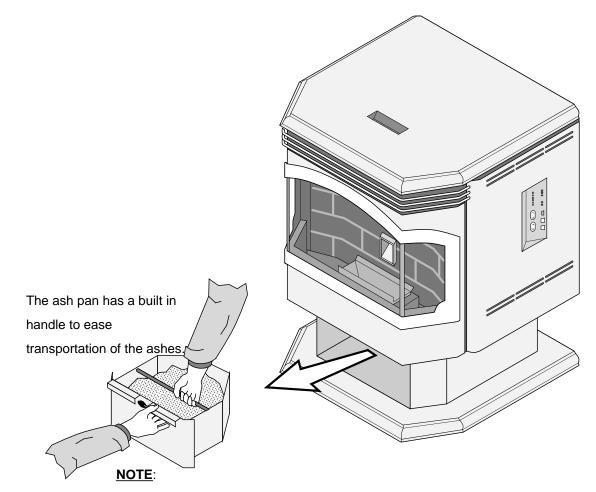
When replacing the ash pan make sure it is pushed all the way in.
