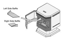
Remove the refractory following the directions below.
