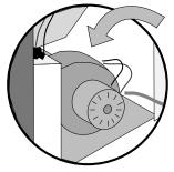
The convection blower inlet can be vacuumed out (if needed). If extensive cleaning is needed, it can be removed for cleaning.
