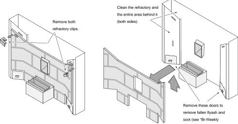
Clean the Exhaust Duct (the stove must be cool and unplugged)
