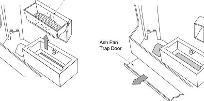
Replace the ash trap doors and firepot. Slide the ash pan trap door forward.
