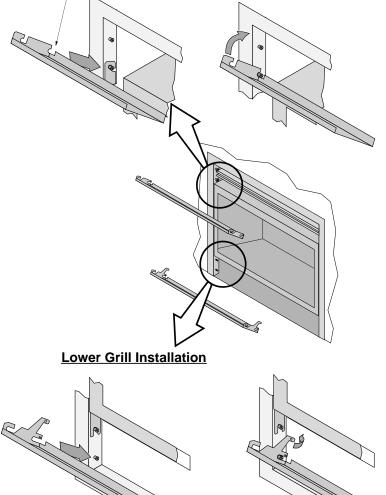
Hold the grill at an angle and insert the lower slot over the bushing on the fireplace (both sides). You may need to press on the grill to get the tab over the bushing (this prevents the grill from accidentally falling off). Bend the tab outward on both sides. This is the end-stop for the lower grill, it allows the grill to swing forward.
