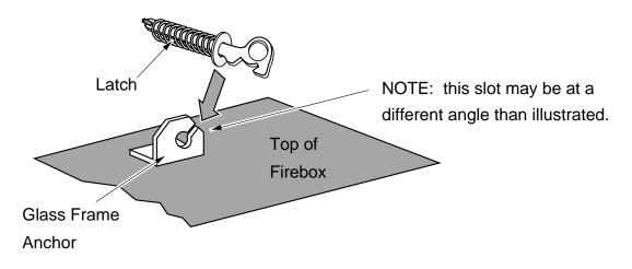
Note how the washer on the latch fits behind the flange on the glass frame anchor.
