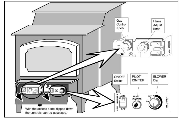
**Blower Knob** This knob controls the speed of the internal convection blower that pushes the heated air into the room.
