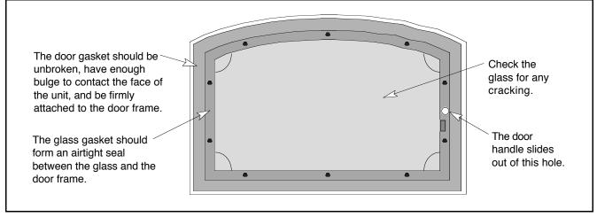
3. Then replace the door. Turn the door handle clockwise until the door seals tight. Tighten the handle until it points downward.
