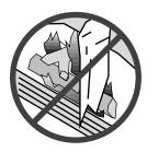
Do not place clothing or other flammable items on or near the heater. Because this heater can be controlled by a thermostat there is a possibility of the heater turning on and igniting any items placed on or near it.
