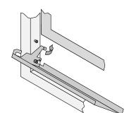
Bend the tab outward on both sides. This is the end-stop for the lower grill, it allows the grill to swing forward.
