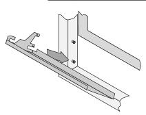
Hold the grill at an angle and insert the lower slot over the bushing on the fireplace (both sides). You may need press on the grill to get the tab over the bushing (this prevents the grill from accidentally falling off).
