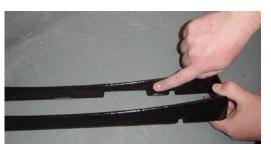
4 Remove the four screws securing the glass tray. Lift the tray up and place it aside.
