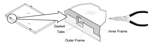
**REMOVAL INSTRUCTIONS**: carefully bend the tabs out with needle-nose pliers (there are tabs on the inner and outer frame - the center tabs only have tabs on the inner frame). <u>Do not pry these tabs, this may cause the glass to crack</u>.
